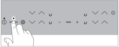
When the "Stop+Go" sensor panel is actuated again, the cooking settings that were previously selected are reset and the control light goes out.
